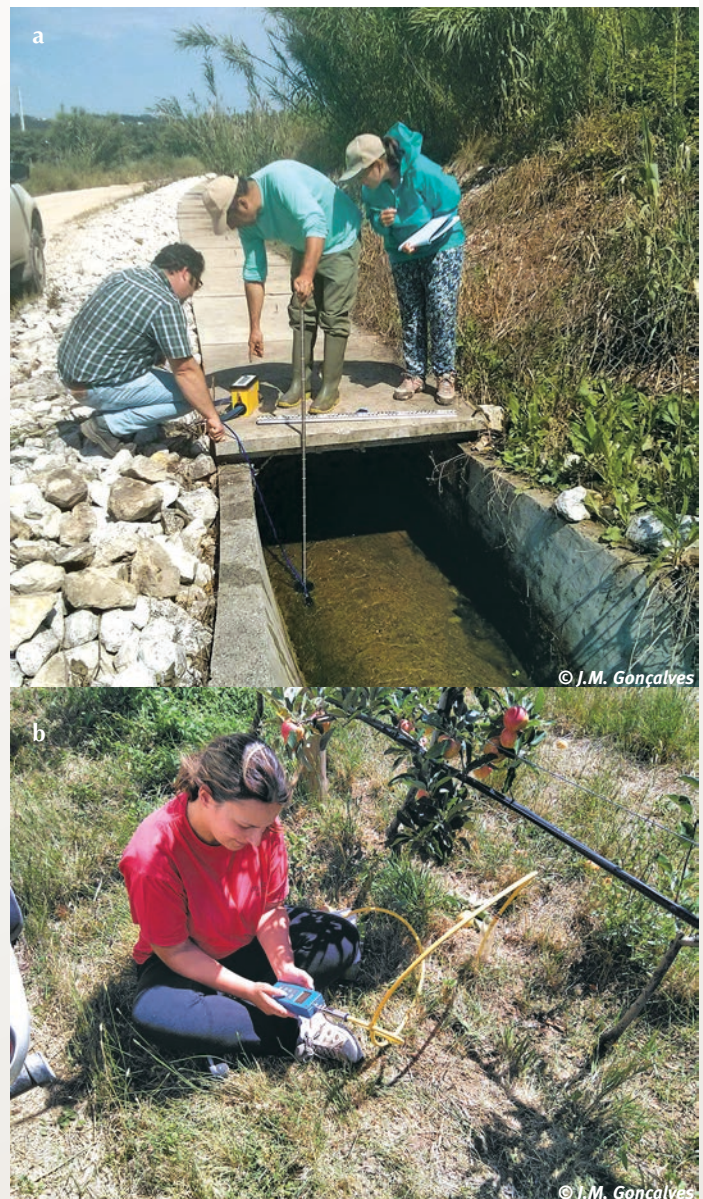
View of field monitoring activities: a) canal flow rate with electromagnetic current meter; b) soil moisture with TDR.
