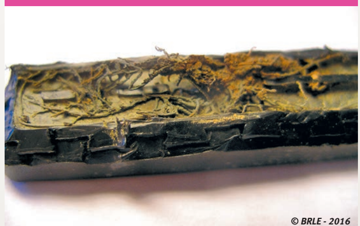
2 Root intrusion in a dripper in a peach orchard.
